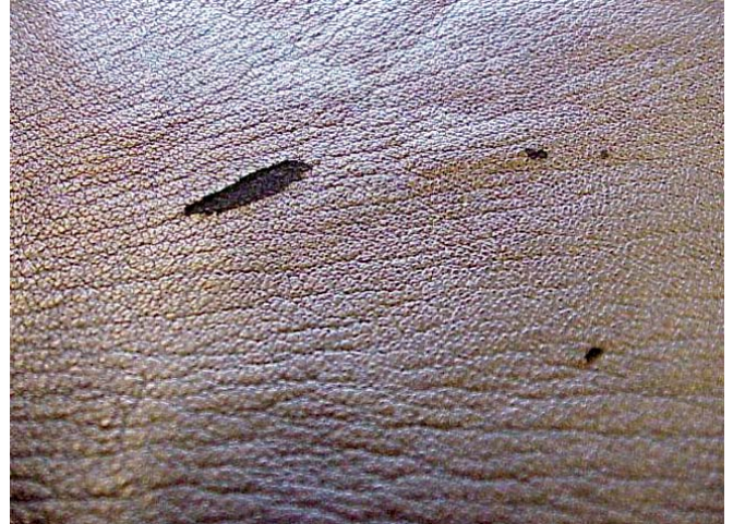
Scratch damage is magnified on the distinctive grain of finished deer leather. This has been identified as the main quality issue for the leather industry.
